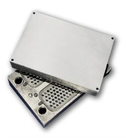
Subsequently, all capillaries are checked and calibrated to get a perfect homogeneity along the entire working width of the spinneret.
